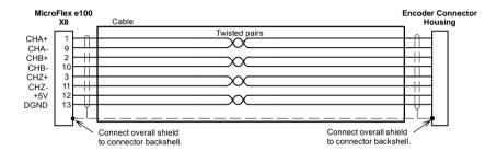
Figure 54 - Encoder signal cable grounding
